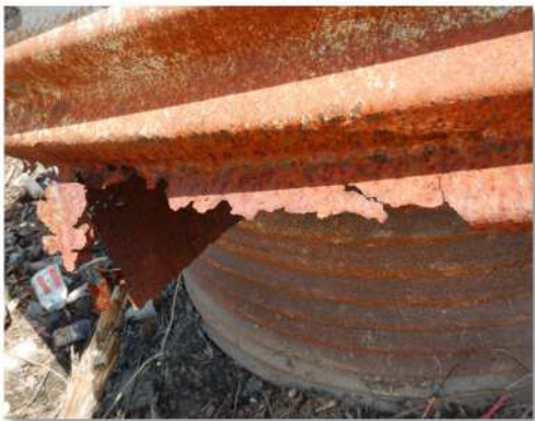
Pic. 2. Highly corroded riser leaning on one side.
