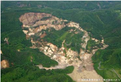
A large-scale landslide in the upstream basin of the Aratogawa reservoir, caused by the Iwate-Miyagi Nairiku earthquake occurred in 2008.
