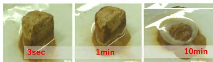
Figure 10 Failure in Water
