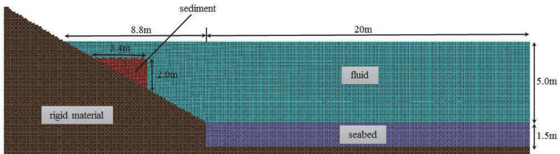
Fig. 3 Configuration of particles at 0.0 sec of case2
