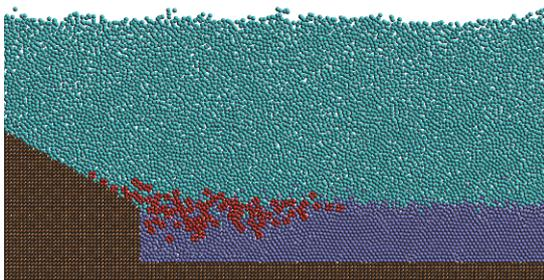
Fig. 6 Configuration of particles at 60.0 seconds when the density of the sediment is equal to the floating mud
