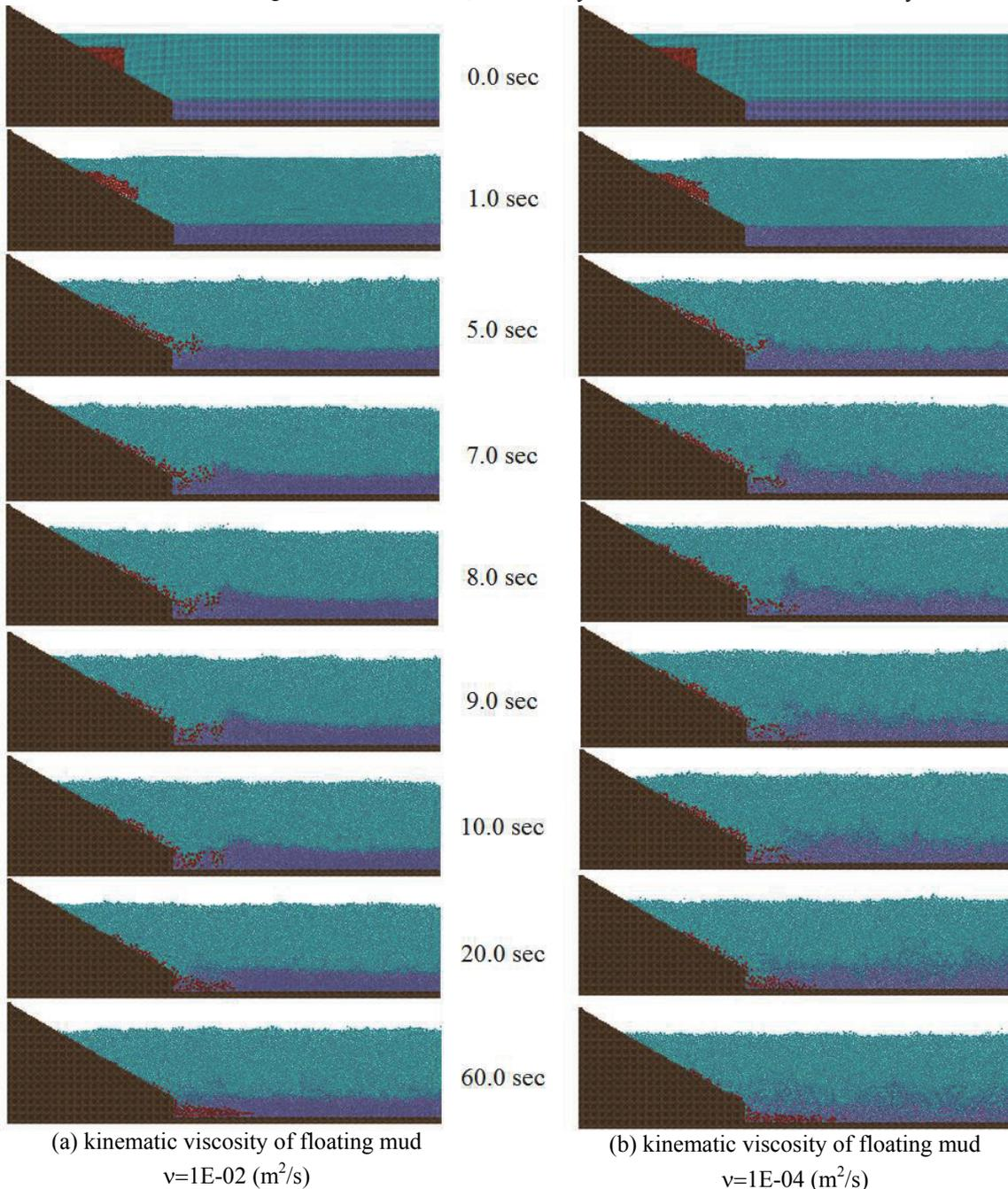
Fig. 5 Configurations of particles from 0.0 seconds to 60.0 seconds of case2
