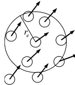
Fig. 1 Concept of the particle interaction model in MPS
