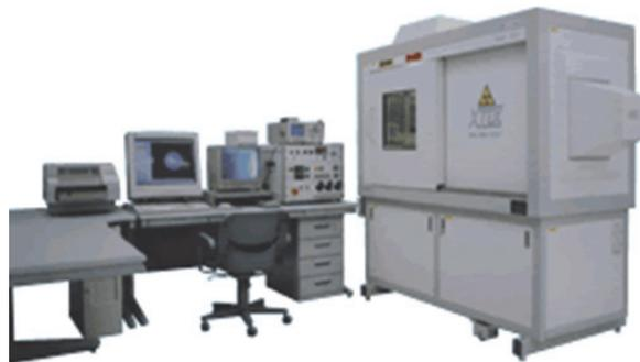
**Fig.2** Micro focus X-ray system assembled by TESCO Corporation
