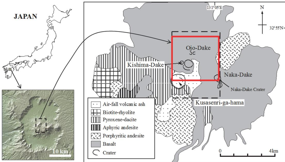
Fig. 2 The locations of Aso Volcano and the GREATEM survey area. Dashed and red rectangles are the flight area and the survey area shown in Fig. 3, respectively.
