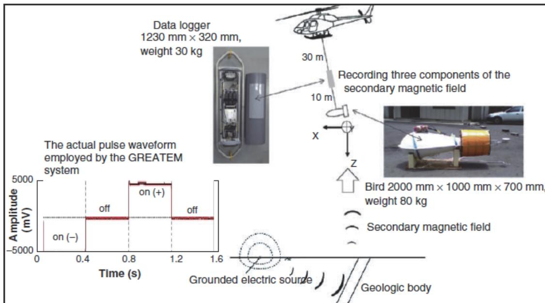
Fig. 1 Overview of the GREATTEM system. The towed bird contains the three-component magnetometer, gyro, directional MI sensor and GPS sensor. The data logger has a 24-bit AD converter, SSD memory, and a high-precision clock synchronized with the transmitter-control clock in the towed container. The secondary magnetic field induced in accordance with the ground resistivity is recorded during current 'on' and 'off' times.
