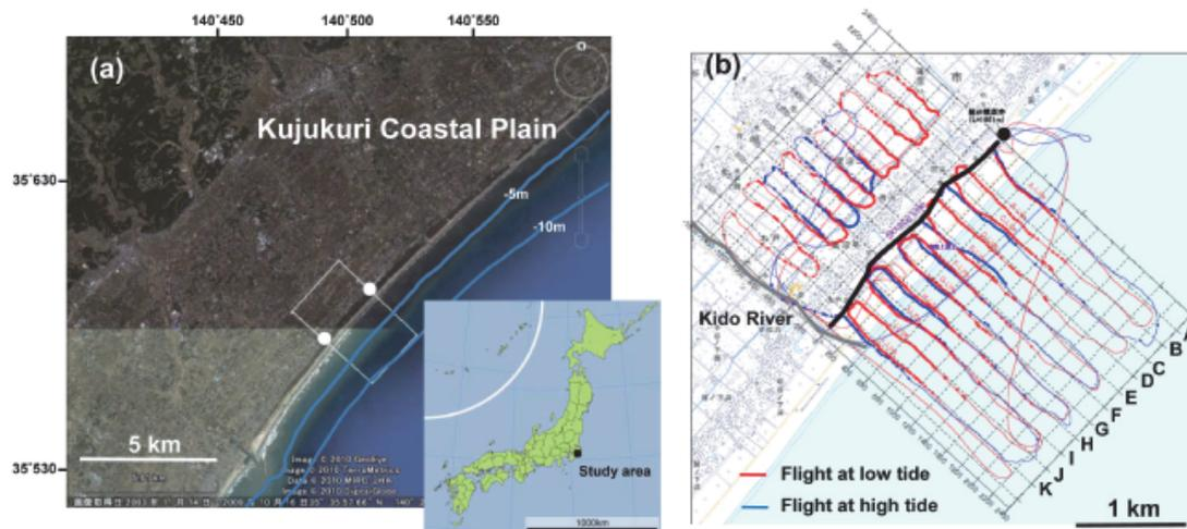
Fig. 4 (a) Location of survey area in the Kujukuri coastal plain with 5-m bathymetric contours. White dots denote the places where current dipole electrodes were placed. (b) Survey area and flight lines. The thick black line indicates the transmitter cable, which was placed 300–400 m inland and parallel with the coastal line. Meaningful data were obtained along flight lines with a thicker color. A black dot indicates the wellbore site in Hayashi et al. (2009).
