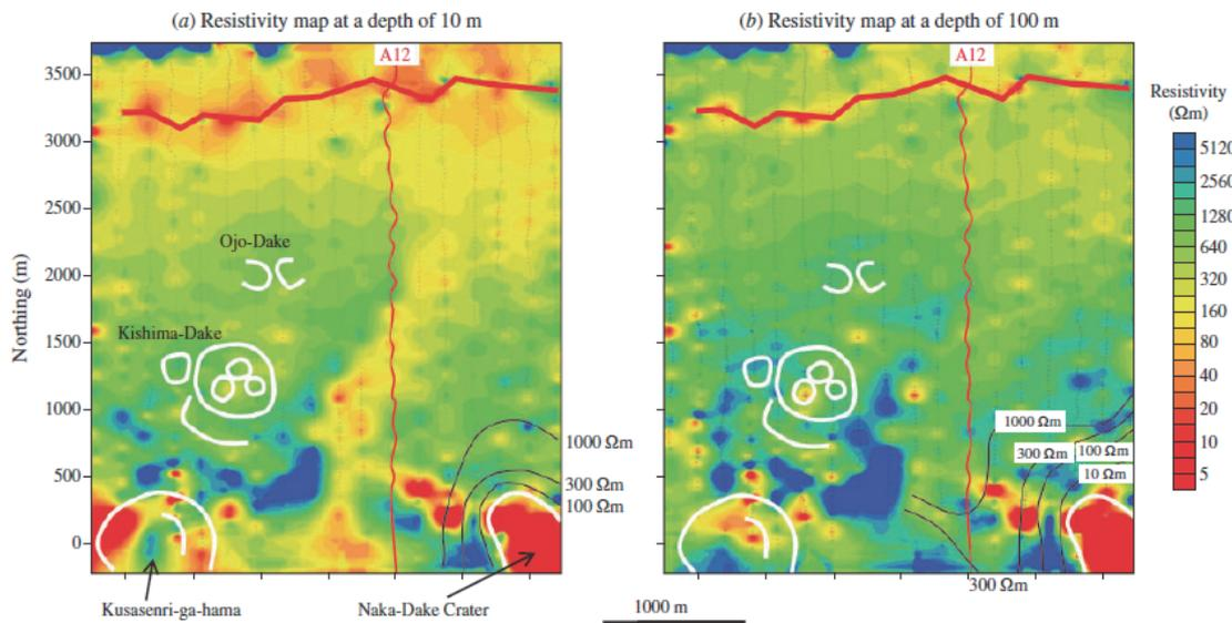
Fig. 3 Resistivity maps at depths of 10 m (a) and 100 m (b) using data from a flight height of 100 m in 2004. The thick red line indicates the transmitter cable (electrical source). The location of flight line A12 (thin red line) is shown for reference. White lines indicate the craters. Resistivity contours (a) and (b) are those at ground surface and at 1000 m elevation (corresponding to ~100–250 m depth) in Handa and Tanaka (1999), respectively.
