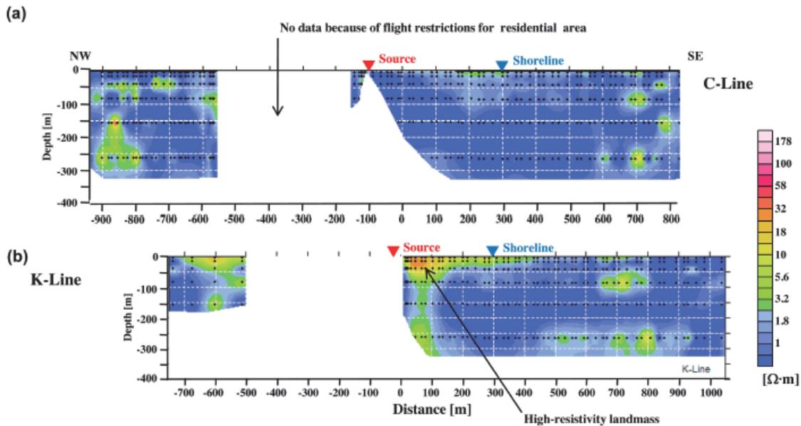
Fig. 5 Resistivity profiles along flight lines C (a) and K (b) at low tide.
