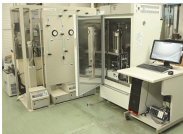
Photo 1 Test apparatus for two-phase flow experiments using supercritical CO 2
