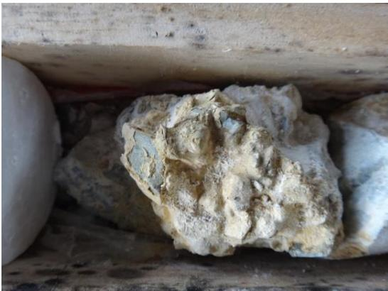
Photo. 3 Dissolution of borehole core drilled at lining concrete
