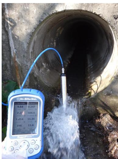
Photo. 2 A water quality measurement device (temperature, pH, EC, Eh)
