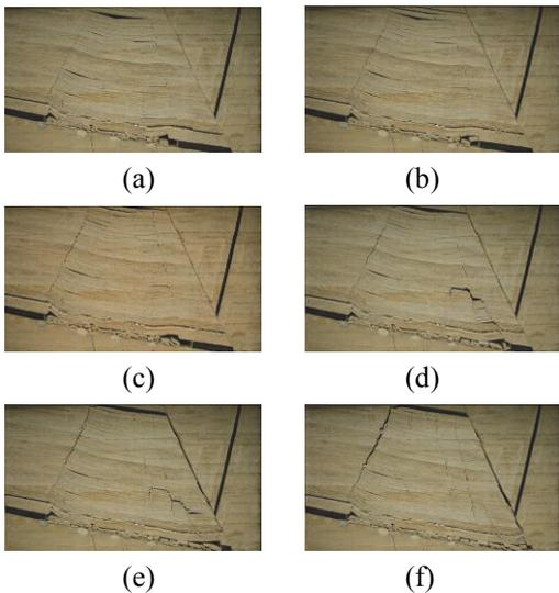
Fig. 6 Overburden deformation and failure situations at each stage
