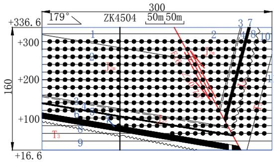
Fig. 2 Engineering geological model of profile Line.45
