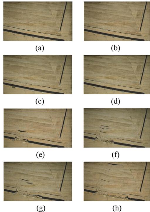
Fig. 4 Overburden deformation and failure at different stages
