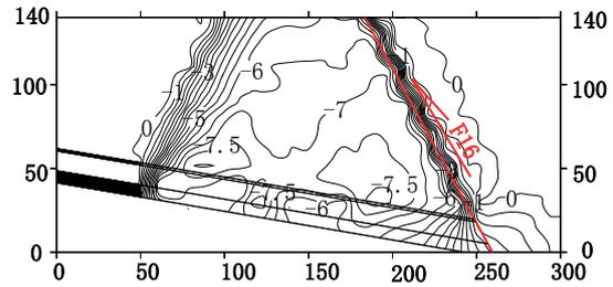
Fig. 7 Contour map of roof subsidence after mining without setting up fault coal-pillars
