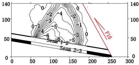
Fig. 5 Contour map of roof subsidence after mining when setting up fault coal-pillar
