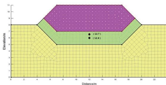
Fig. 2 Grid division for generalized model of Yanqun landfill site
