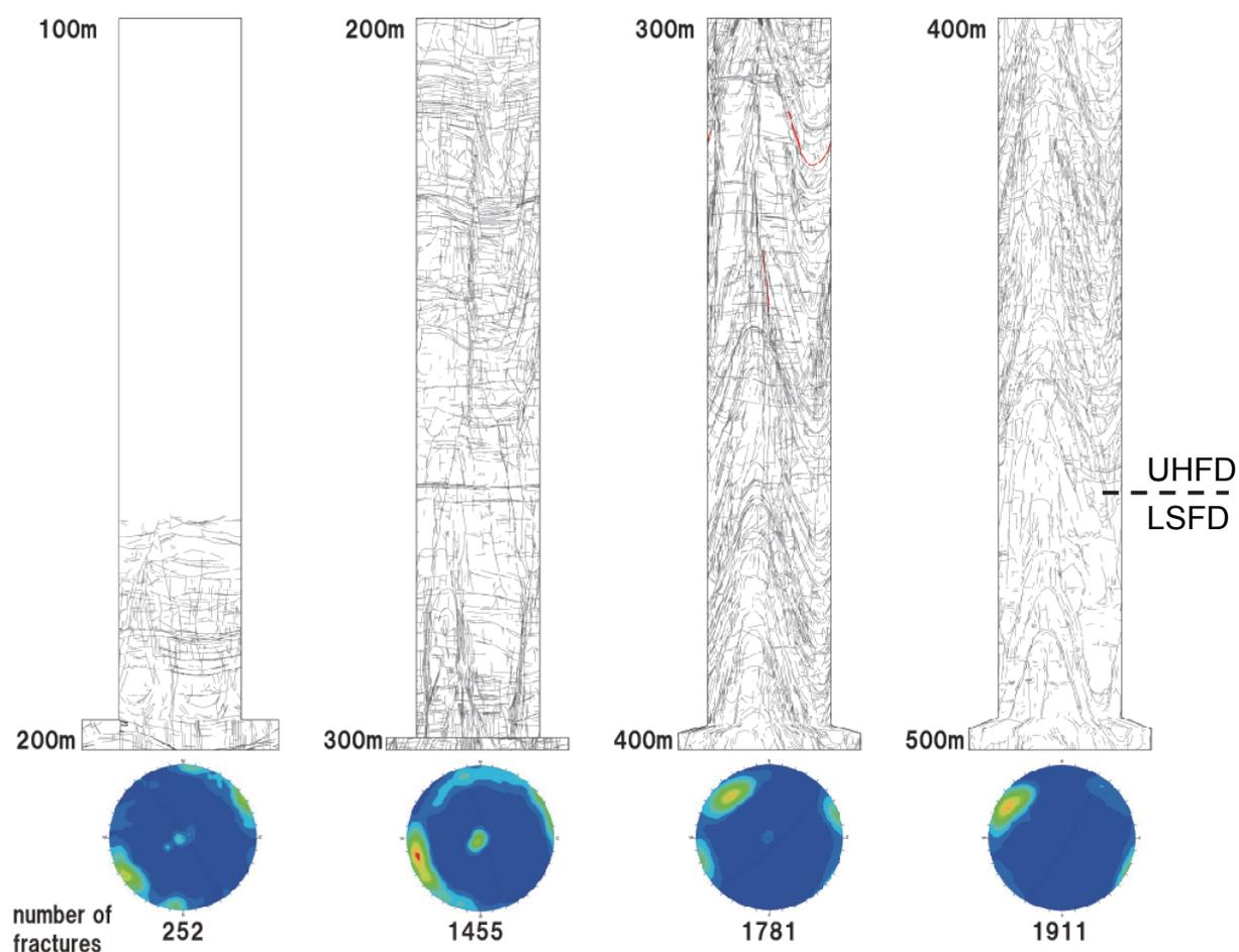
Fig. 2 Sketch map of fracture distribution within the ventilation shaft (development view of shaft wall), and Schmidt stereonet diagrams showing fracture orientations (lower hemisphere projections of poles to fracture).
