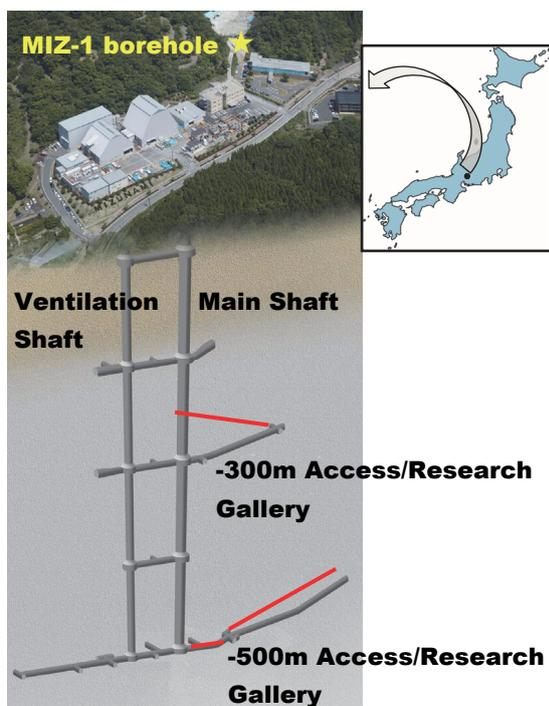
Fig. 1 Location and facility allocation of the Mizunami Underground Research Laboratory (MIU). Red lines indicate the location of boreholes examined, and yellow star indicates the location of MIZ-1 borehole referred in Figure 4.
