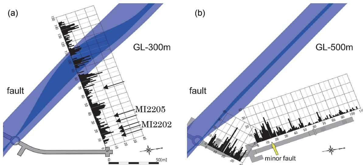
Fig. 3 Density of fractures confirmed by borehole investigation at two different level. (a) at the GL-300m, and (b) at the GL-500m.
