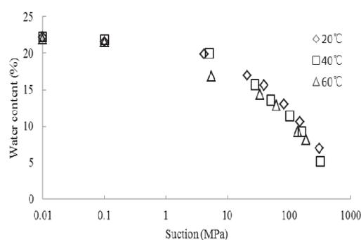
Fig. 3 Influence of temperature on water retention properties (initial dry density 1.90g/cm<sup>3</sup>)
