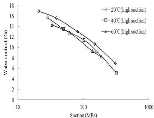
Fig. 4 Influence of temperature on SWRCs of GMZ01 bentonite at high suctions ( $1.90\text{g}/\text{cm}^3$ )
