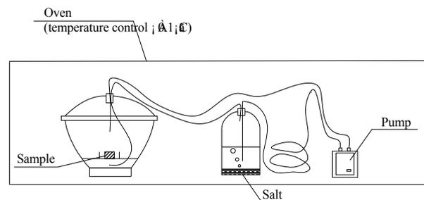
Fig. 1 Setup for the vapour equilibrium method with temperature control (Ye et al., 2012)
