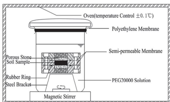
Fig. 2 Setup for the osmotic technique with temperature control (Ye et al., 2012)
