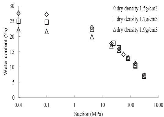
Fig. 5 Influence of dry density on water retention curves ( $20^\circ\text{C}$ )
