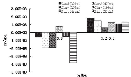
Fig.9 Comparison of the resilient modulus of different soils in repeated spring-back process with 3.2~2.8MPa
