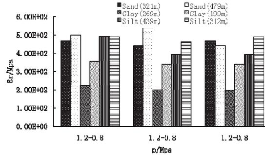
Fig.7 Comparison of the resilient modulus of different soils in repeated spring-back process with 1.2~0.8 MPa
