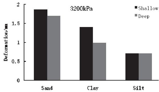
Fig.5 Comparison of the deformations of different soils under 3200 kPa
