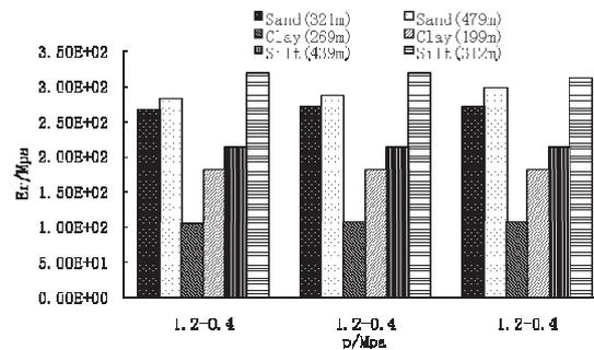
Fig.8 Comparison of the resilient modulus of different soils in repeated spring-back process with 1.2~0.4MPa
