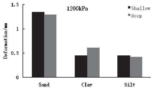
Fig.4 Comparison of the deformations of different soils under 1200 kPa
