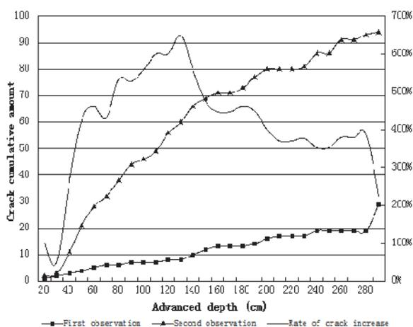
Fig.7 2# borehole camera observation hole result
