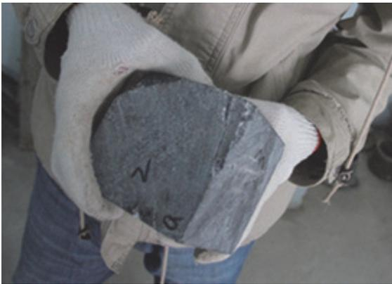
Photo.5 Wedge and crack damages of Sample No. 2 after the first stage 1-1a, 4<sup>th</sup> round of stress rotation test
