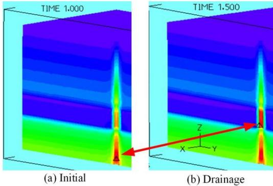
Fig. 7 Location change of maximum shear stress in shaft lining
