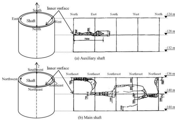
Fig. 4 Failure sketches of two shafts
