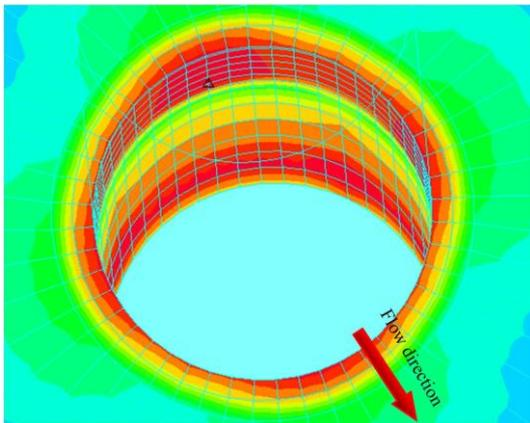
Fig. 8 Maximum shear stress condition during drainage
