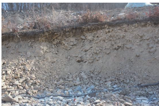
Fig. 6 Yellow colluvial deposit consisting of rock blocks and rubble with silty clay filling in interspaces
