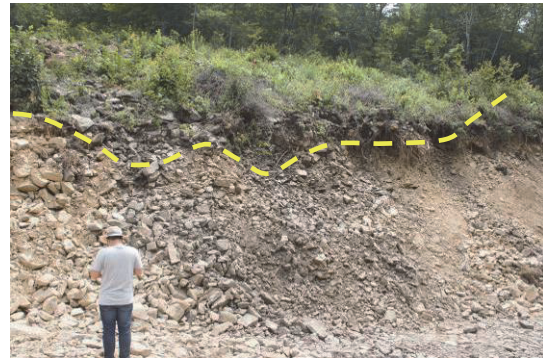
Fig. 7 Rock piles lying over colluvial deposit.
