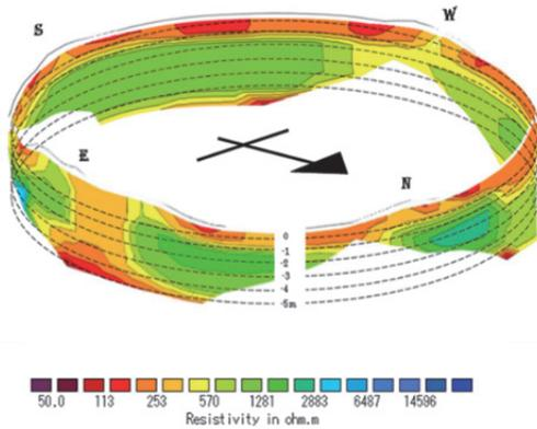
Fig. 10 A bird's eye view of the schematic resistivity profile image beneath the gallery surrounding the central tower obtained from analysis of the Wenner's array
