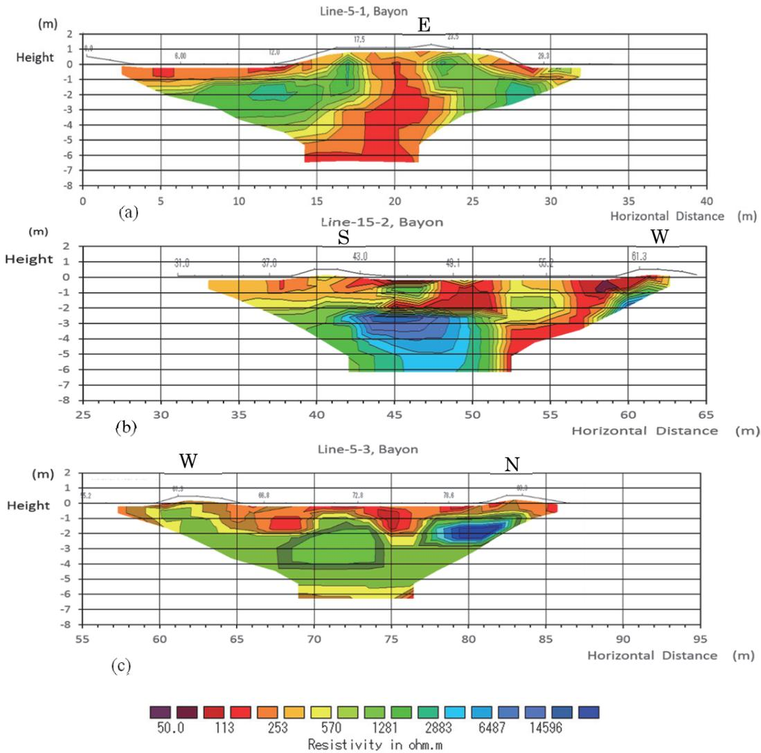
Fig. 7 Resistivity profile (a): Line-1, (b): Line-2, (c): Line3
