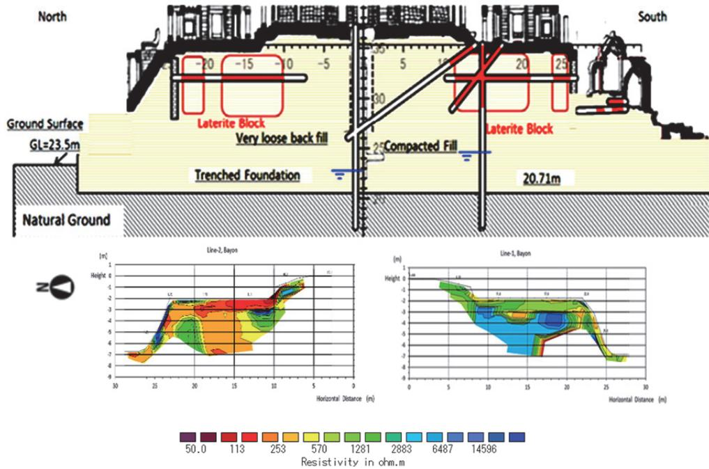
Fig. 9 Comparison between the geological section and the resistivity profile under upper terrace of the Bayon temple
