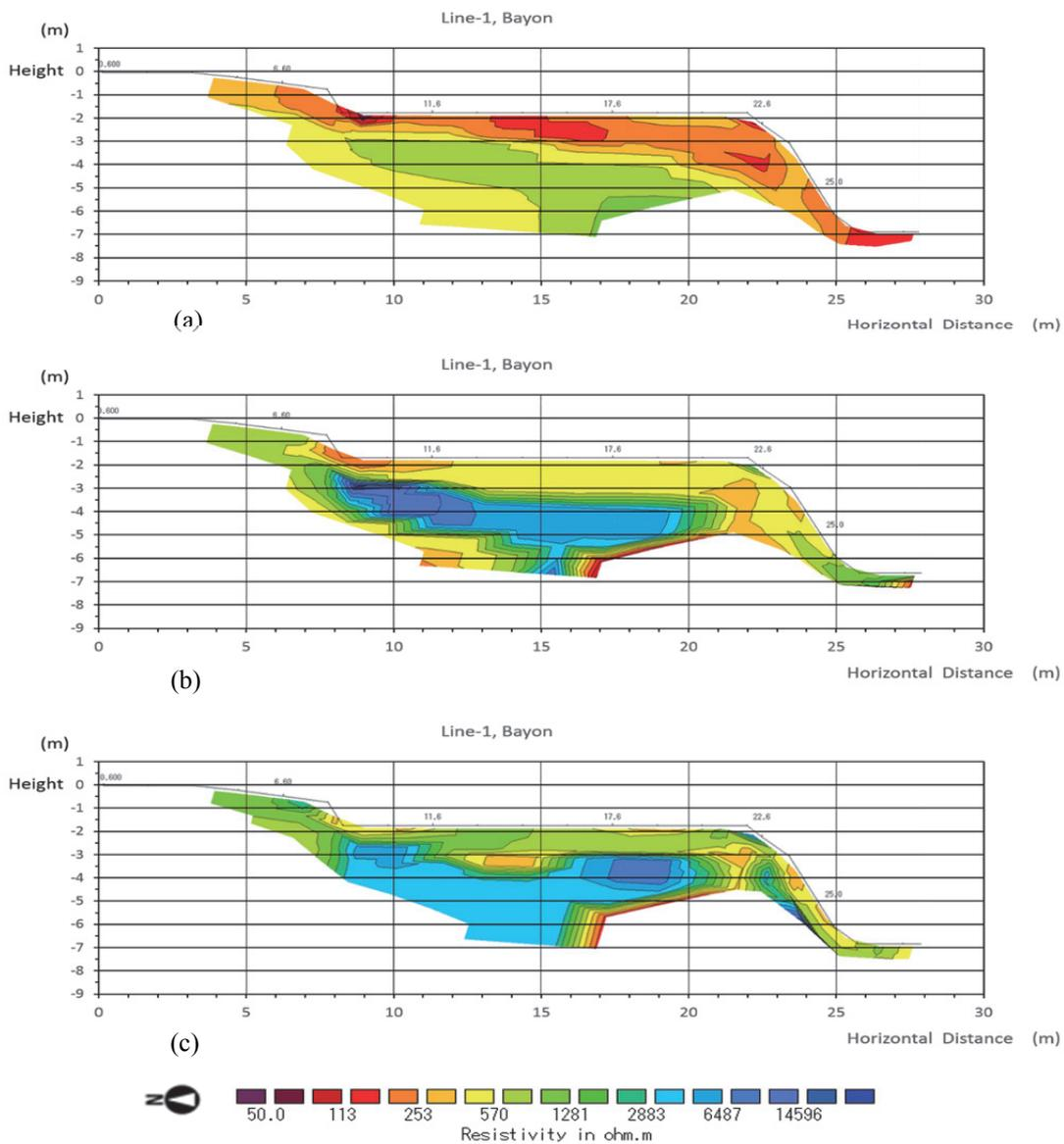
Fig. 5 Resistivity profiles determined from the different measurement methods
