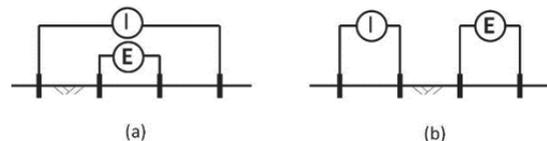
Fig. 3 Electrode array of typical four poles technique
