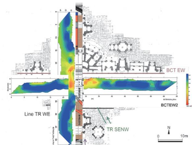
Fig. 11 Resistivity profiles of the N-S and E-W lines (from Nakagawa et al., 2012)
