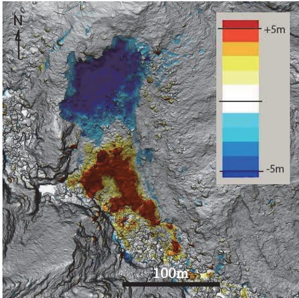
Fig.7 Distribution of altitude change after debris slide. Blue areas show the locations where the altitude was 5 m lower, while red areas show the locations where the altitude was 5m higher after debris slide.
