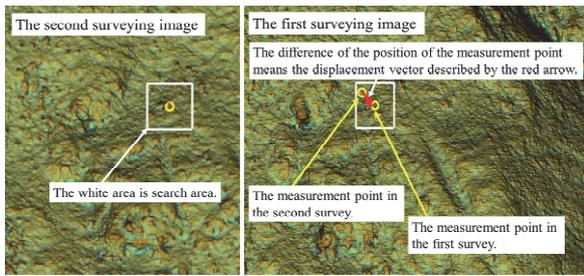
Fig. 4 Matching method for image. The amount of movement of the measurement point represented by the yellow circle is computed using the first and second surveying images. The white square is specified as the search area in the second surveying image and in the first surveying image. The same point in the first and second images is specified as the measurement point using the angle of inclination and the degrees of ups and downs.
