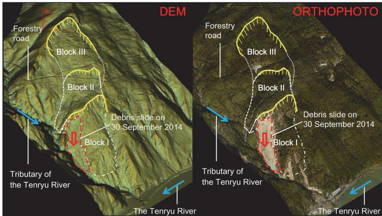
Fig. 5 Bird's eye view image of the landslide area produced from DEM and Orthophoto data
