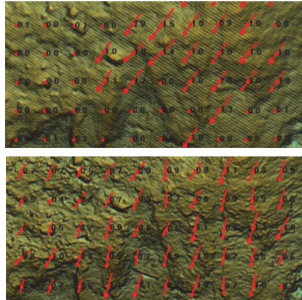
Fig.8 Distribution of displacement in the area where debris slide occurred. The upper figure show the analysis result by using all laser point group data. The lower figure show the result by our proposed method.
