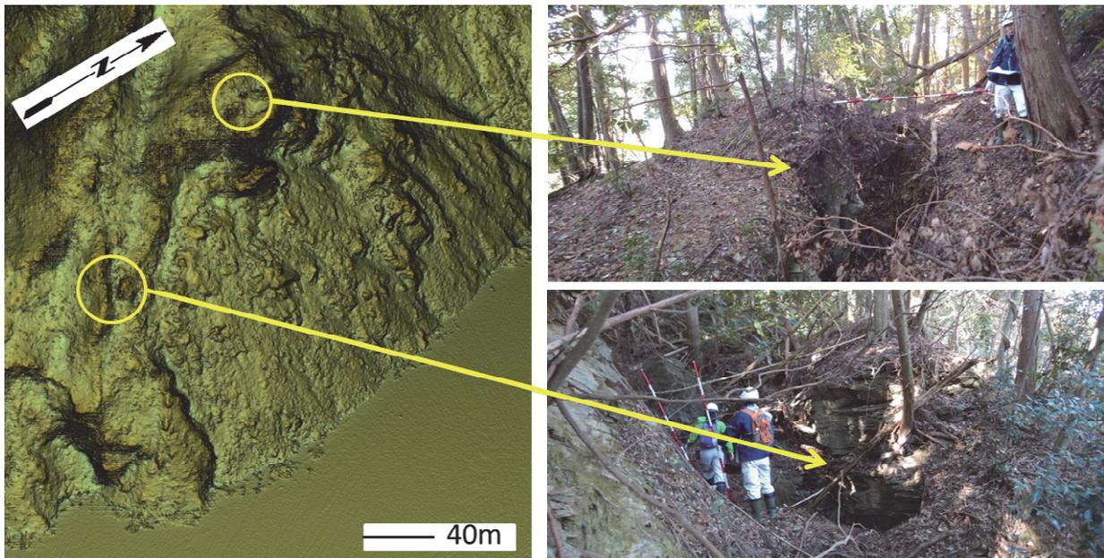
Fig.3 Example of reading the detailed land features using the method shown in Fig.1. It was possible to read 2 m deep concave topography and 3 m wide tub-shaped topography.
