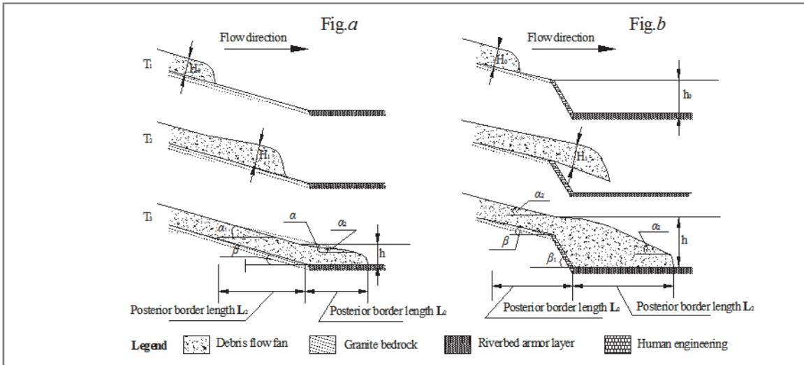
Fig.12 Two classifications of deposit fans model
