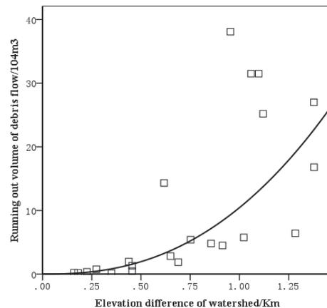
Fig.7 Empirical relationship between the landslide volumes and elevation difference
