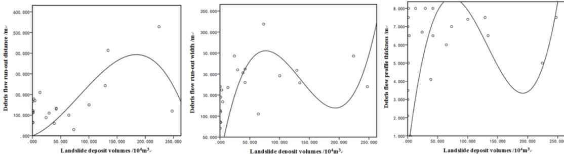
Fig.10 Empirical relationship between deposit features and landslide deposit volumes
