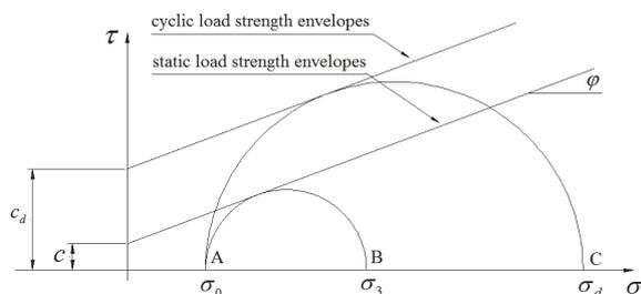
Fig. 7 Mohr-circle and failure envelope under static and dynamic load
