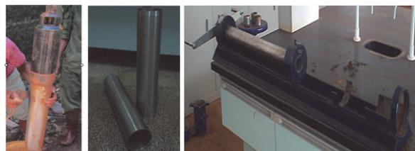
Fig. 1 Undisturbed soil field sampling equipment and horizontal bulldozing
