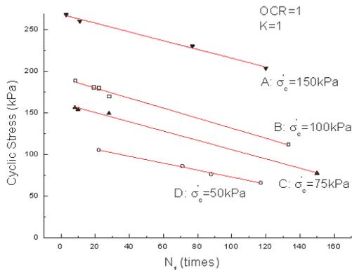
Fig. 6 Dynamic Shear stress - failure vibration time curve
