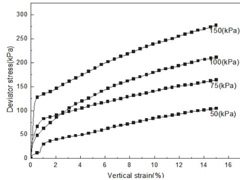
Fig. 4 Stress-strain curve under cu static
