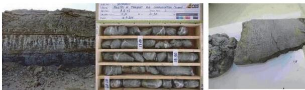
Photo 6: Green clays associated with Ancient sabkha in sections and bore hole cores- port area
