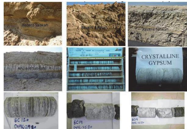
**Photo 4: Exposed sections and in cores recent & sub-recent sabkha in Port area**
