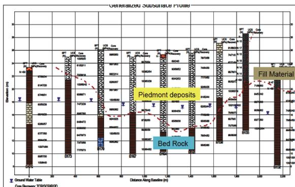
Fig. 4: Geological sections showing the bed rock / green clays at depth underlying the piedmonts.
