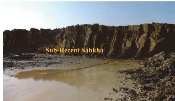
**Photo 3: Exposure of sub-recent sabkha in excavations - Port area**
