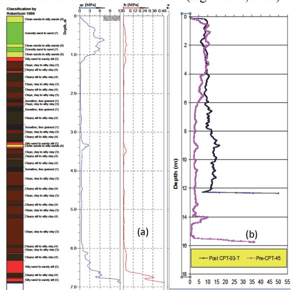
**Fig. 6: Typical CPT plots showing (a) qc, fr & soil type with depth (b) degree of ground improvement in fills.**
