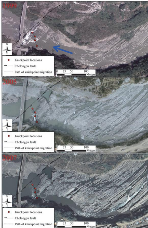
Fig. 2 The knickpoint locations are identified on a series of aerial photographs (the Pifong Bridge of the Tachia River).
