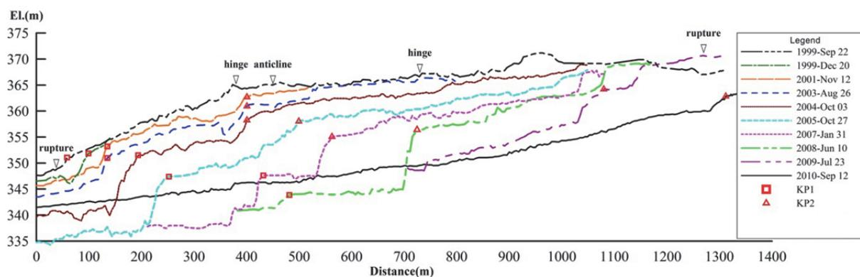
Fig. 3 The longitudinal profiles derived from DEM data for knickpoint locations identification (the Taan River).
