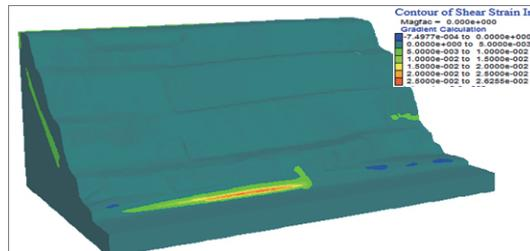
Figure 18 Slope shear strain increment nephogram after cutting slope
