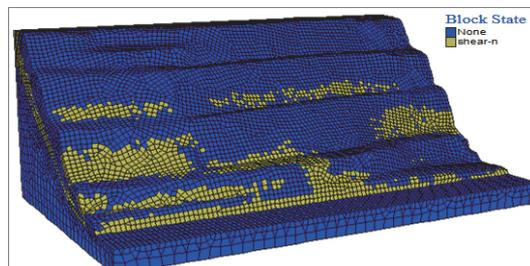
Figure 19 Slope plastic zone map after cutting slope
