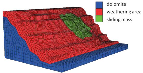
Figure 7 3D model of 2# slope of Baiyun'ebo
