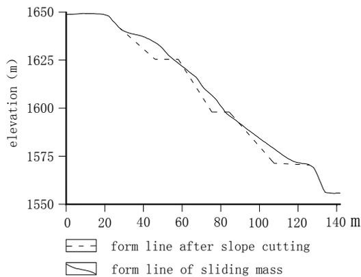
Figure 15 Typical profile before and after treatment of landslide
