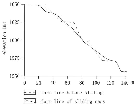
Figure 3 Profile of 2# slope in D area of main mine
