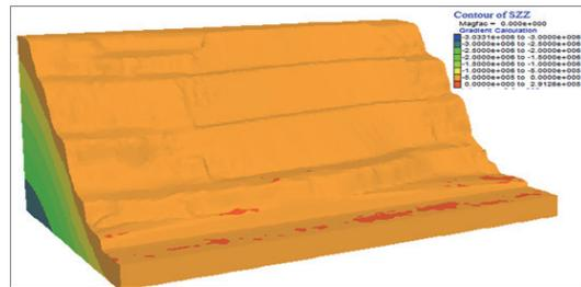
Figure 17 Slope stress distribution nephogram after cutting slope
