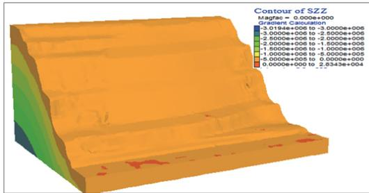
Figure 9 Slope stress distribution nephogram before sliding
