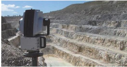
Figure 6 three dimensional laser scanner
