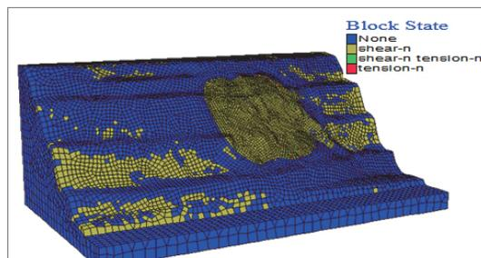
Figure 14 Slope plastic zone map after sliding
