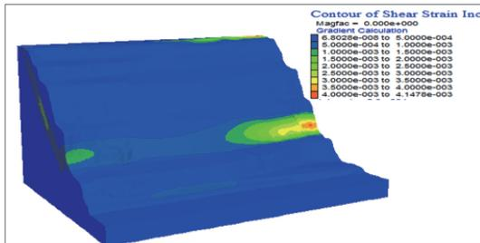
Figure 10 Slope shear strain increment nephogram before sliding
