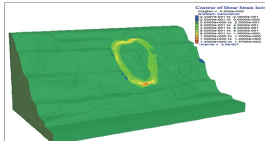
Figure 13 Slope shear strain increment nephogram after sliding
