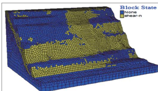
Figure 11 Slope plastic zone map before sliding
