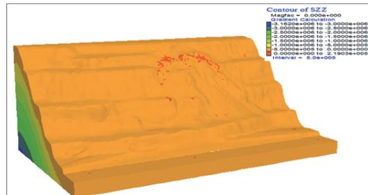
Figure 12 Slope stress distribution nephogram after sliding
