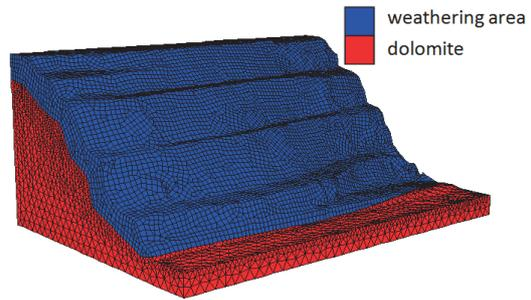
Figure 16 3D model of slope terrain after cutting slope
