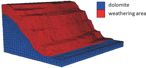
Figure 8 3D model of Slope terrain before sliding
