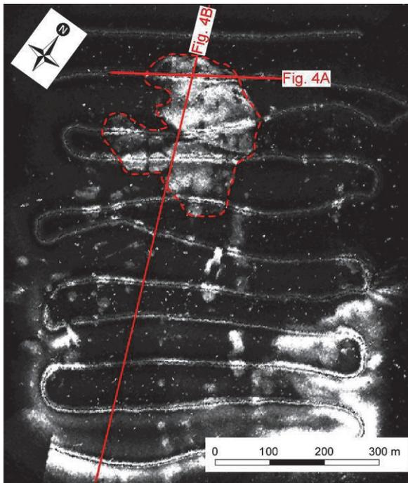
Fig. 3 Synthetic side-scan sonar images indicated in Fig. 2. Red dashed line enclosed area is "high reflection area".
