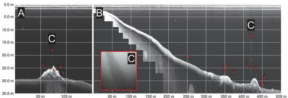
Fig. 4 (A and B) Vertical acoustic profiles of 455 kHz shown in Fig. 2 and 3. Red arrows indicates trees standing on the lake floor. (C) A trunk of tree observed by underwater camera.
