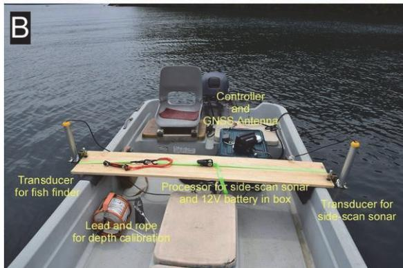
Fig. 1 (A) Schematic diagram of the fish-finder system and (B) photo of the boat equipped with the transducers. Further details are suggested in the text.
