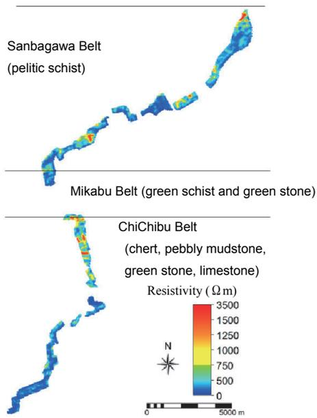
Fig. 2 Resistivity distribution in the three different geological belts.
