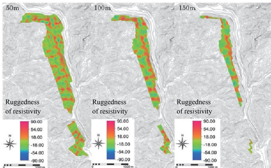
Fig. 3 Ruggedness of resistivity with different radial distance; 50m, 100m 150m
