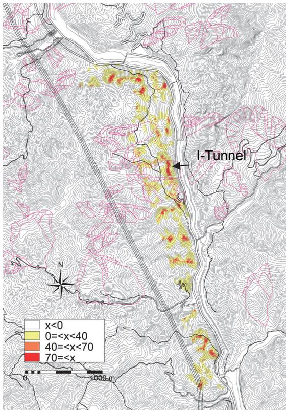
Fig. 4 ISEDCL estimated using the ruggedness of resistivity with 50 m radial distance and topographic effect of amplifying seismic wave, with peak ground acceleration (PGA) 400gal. ISEDCL is categorized into four levels
