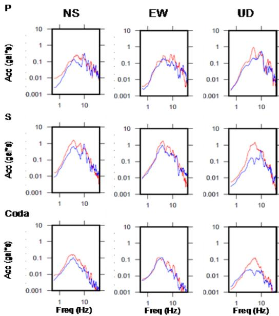
Figure 4: Spectrum of the seismic waveform records on the filled slope (red) and on the sediment ground (blue) for the event on Nov. 29, 2013.
