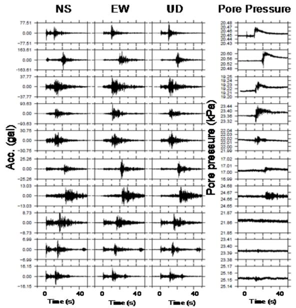
Figure 5: Seismic waveform and pore pressure records on the filled slope for several events whose epicenters are shown in Figure 2. The maximum acceleration was less than 10 gal in the second and third events from the bottom.
