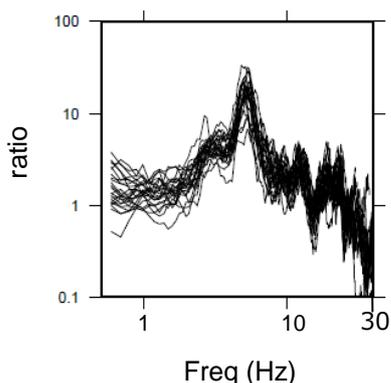
Figure 6: Spectral ratios of updown components for S-waves on the filled slope to those at the sediment ground were shown for all the events analyzed.
