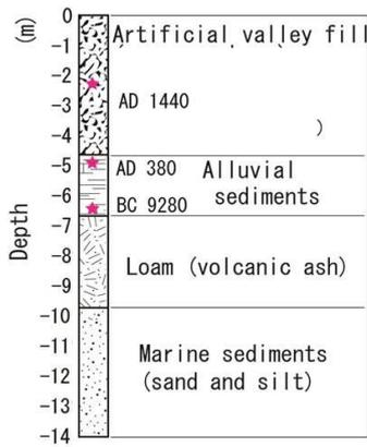
Figure 1: Vertical geological profile in the filled slope at Fusuma-cho Park.
