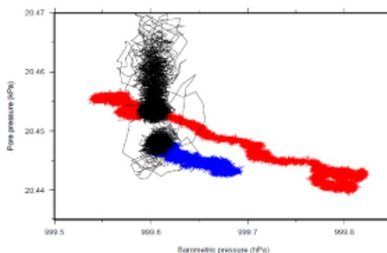
Figure 7: Relationship between barometric pressure and pore pressure during one hour in which the event on Nov. 29 was included. The color shows the time periods: before shaking (blue), during shaking (black), and after shaking (red).
