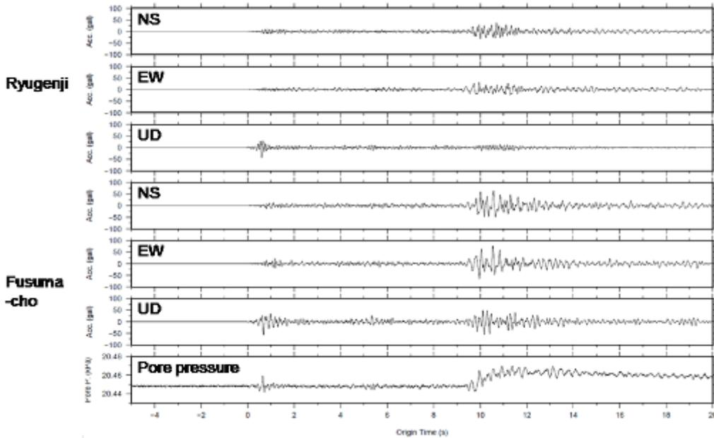
Figure 3: Seismic waveform and pore pressure records for the event on Nov. 29, 2013.
