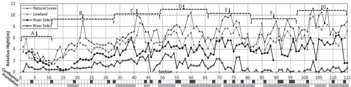
Fig.4 Longitudinal profiles of the Ooyodo River and river conditions relating inundation
