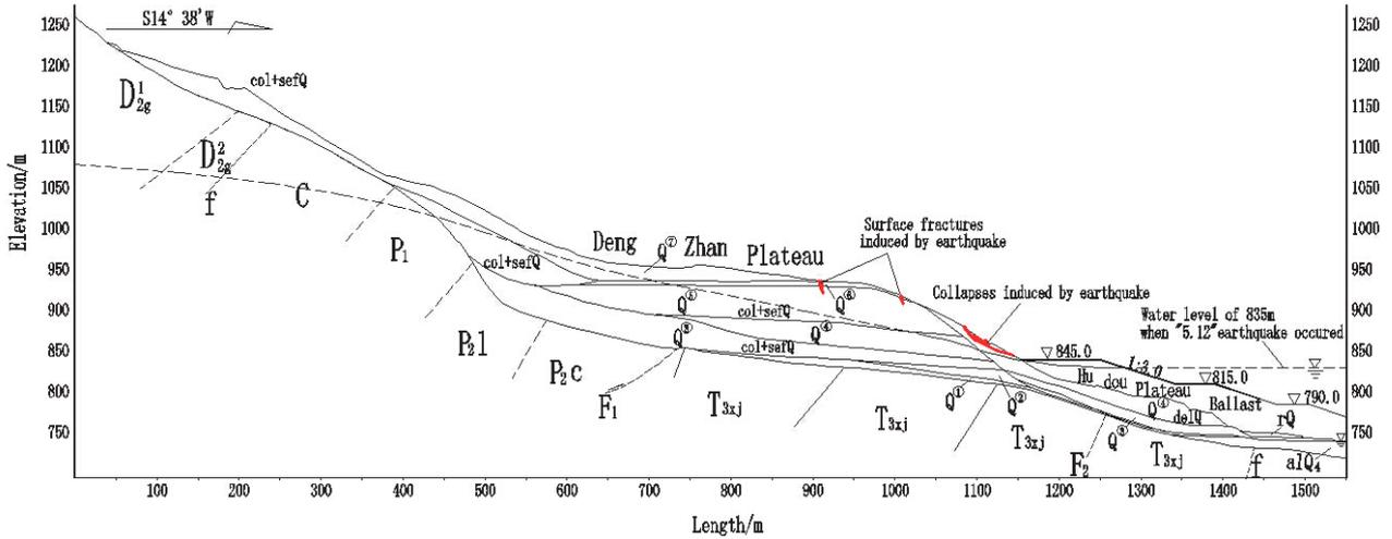
Fig.5 Longitudinal cross-section 1-1 of the talus slope
