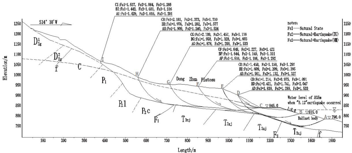
Fig.6 Schematic diagram of calculation cross-section 1-1 of the talus slope under the 835m water level when the earthquake occurred.
