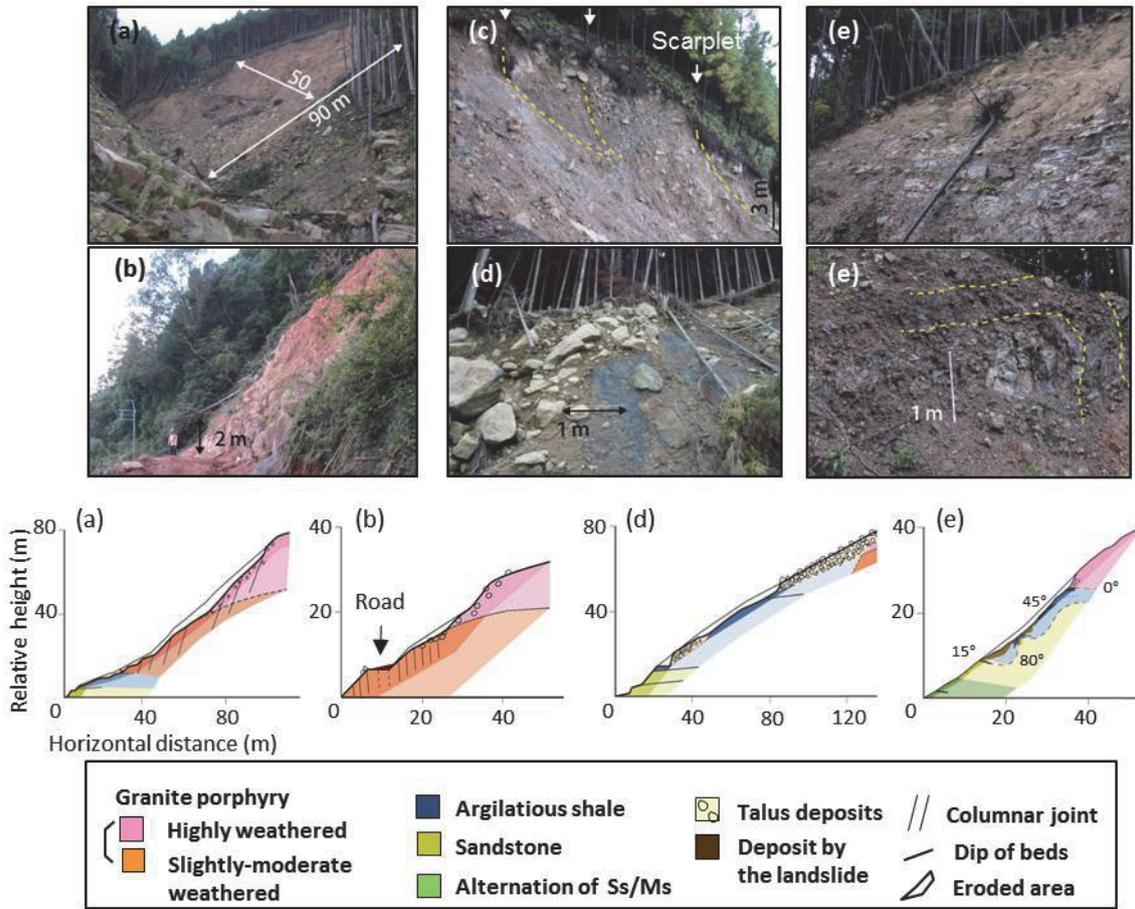
Fig. 7 Photos and cross sections of typical source areas in Nachikatsuura Town in Fig. 6. (a) and (b) Landslides of in-situ weathered granite porphyry. (c) and (d) Those of talus deposit. (e) landslide on a boundary between granite porphyry and sedimentary rocks.
