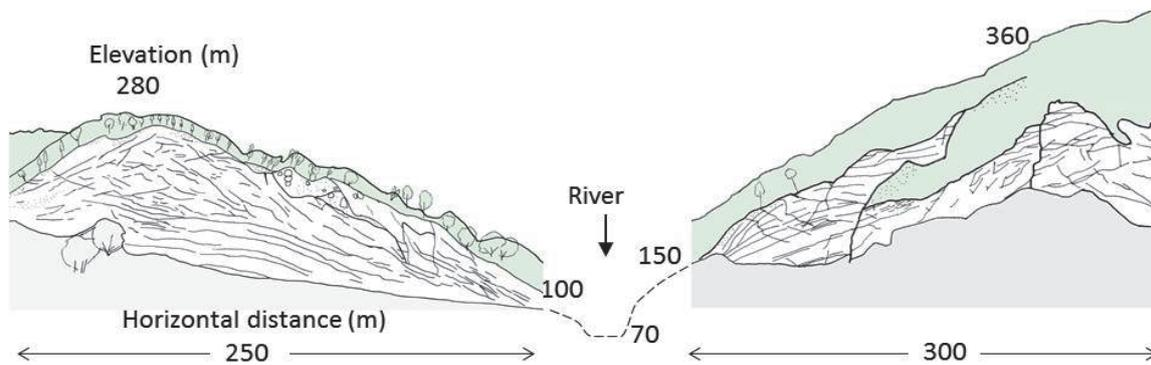
Fig. 2 Sketch of excavation walls of granite porphyry. Most of the narrow lines seem like sheeting joints.
