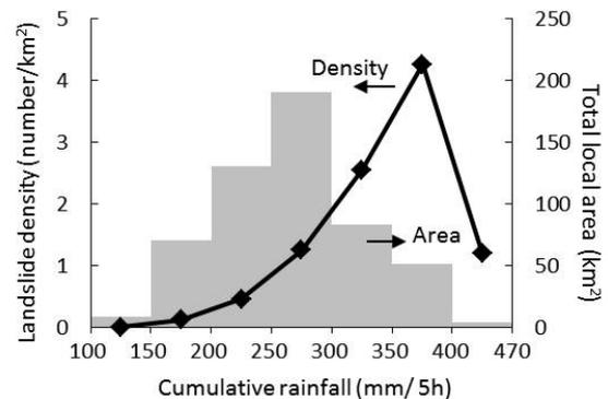
Fig. 5 Landslide densities and total local areas in granite porphyry as a function of the 5 hour cumulative rainfall.
