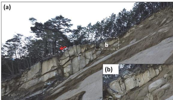
Photo. 2 Right side wall of a landslide scar. (a) Middle-highly weathered rock mass with sheeting joints. The depth of the scar is about 9 m. (b) Close image of the square b.
