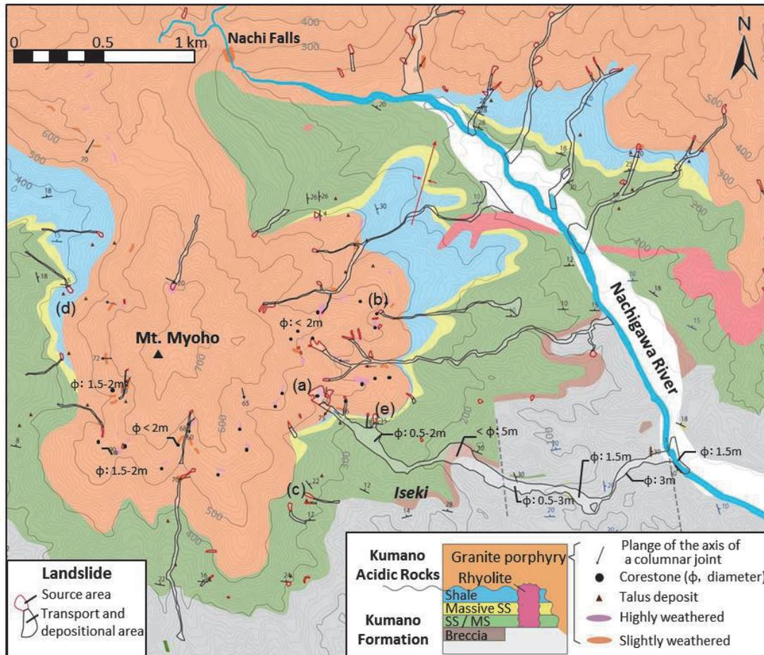
Fig. 6 Landslide distribution on a geological map in Nachikatsuura Town. (a)-(e) indicates the landslide location in Fig. 7. Bedding plains plotted in blue and geological boundaries were modified from Mizuno (1957).
