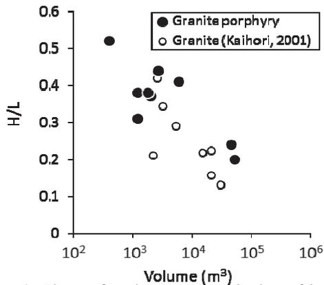
Fig. 8 Plots of volume vs equivalent frictional coefficient (H/L) of landslides.
