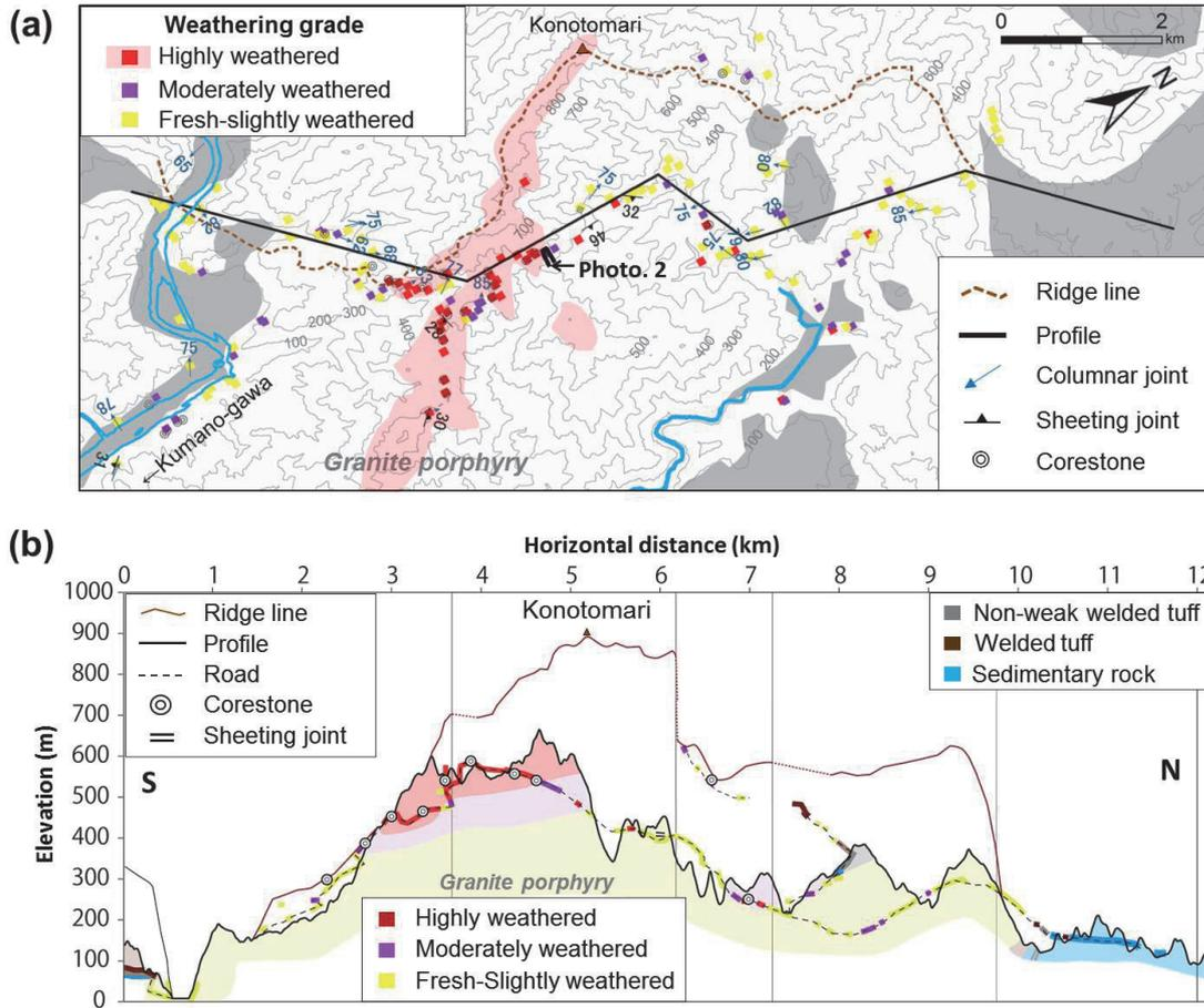
Fig. 3 Weathering mantle in granite porphyry. (a) Plane view. (b) Cross section along the profile line.
