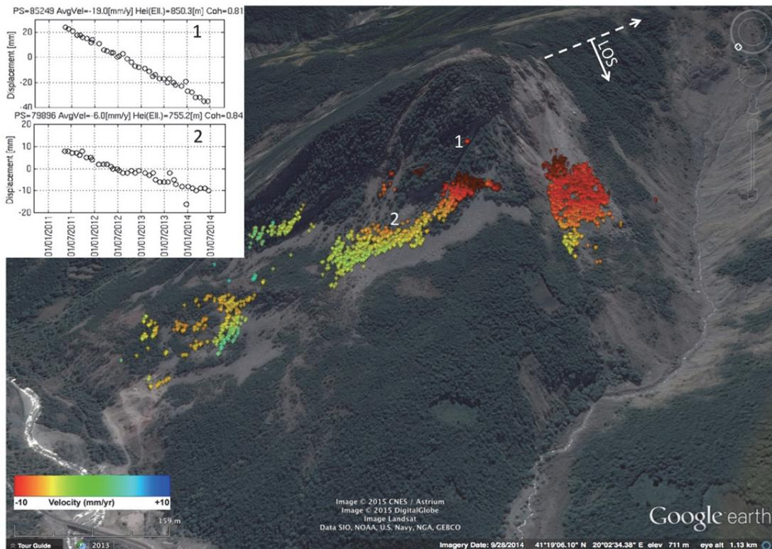
Fig. 3 Unstable slope detected in the mountain range east of Tirana. Reddish to yellowish dots (radar targets) indicate landslide activity and slope deformations and/or instability of slope debris; velocity scale saturated to  $\pm 10$  mm/year. Inset graphs show displacement time series of two representative targets.
