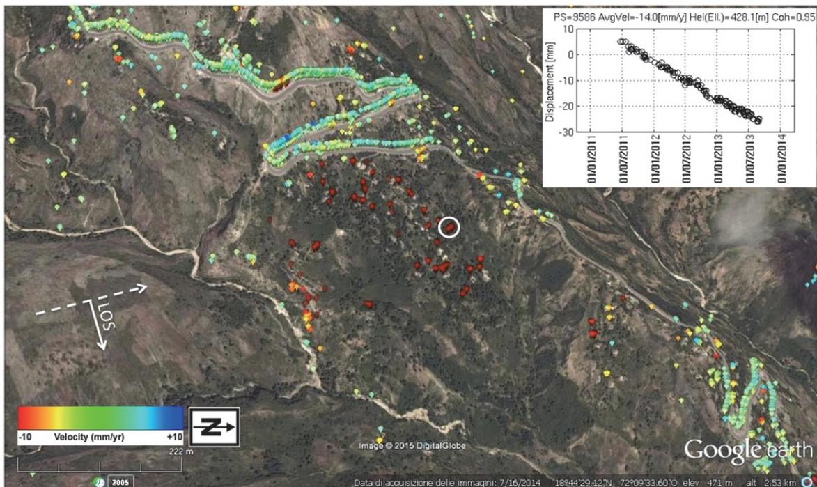
Fig. 5 Deep-seated landslide (center of image) and local instabilities along National Route N°3 of Haiti. Clusters of reddish to yellowish radar targets indicate the landslide motion and localized instabilities affecting the slope and road embankments; velocity scale saturated to  $\pm 10$  mm/year. White circle marks position of landslide target whose displacement time series is shown in inset graph.
