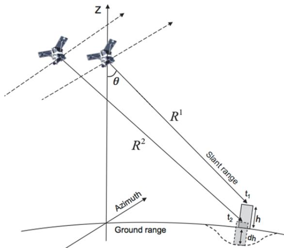
Fig. 1 Two radar acquisitions during successive satellite passes:  $R$  = sensor-target geometrical distance,  $h$  = target elevation,  $dh$  = target displacement, and  $\theta$  = incidence angle (modified after Wasowski and Bovenga, 2014a).
