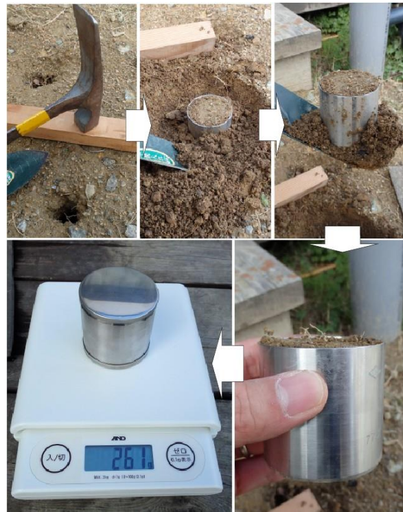
Fig.4 Unit weight test using circular cylinder
