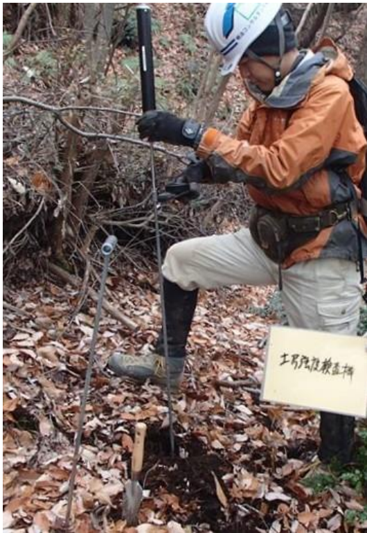
Fig.1 On -site Soil Strength Probe Test (SSPT)
