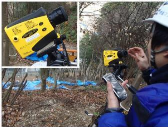
Fig.7 Topographical survey using reflectorless laser measurement tool
