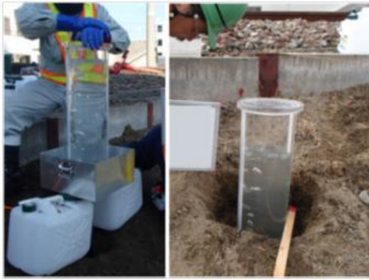
Fig.5 On-site permeability test
