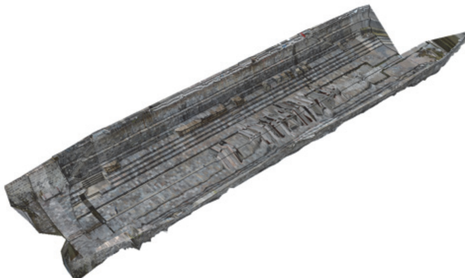
Fig. 4 3-D surface model of the dry dock by photogrammetry
