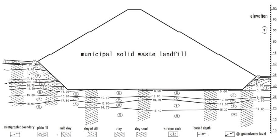
Fig. 1 Soil layer distribution of Yanqun landfill
