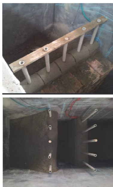
Fig.2 Fabrication of goafs
