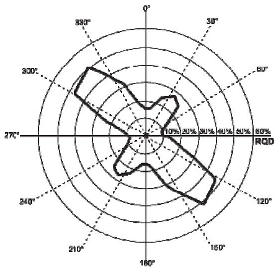
Fig.5 RQD in all directions on tunnel cross section
