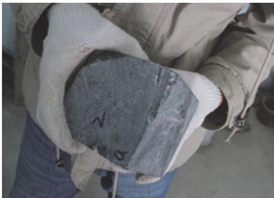
Photo.5 Wedge and crack damages of Sample No. 2 after the first stage 1-1a, 4<sup>th</sup> round of stress rotation test
