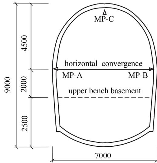
Fig.4 Measuring points for displacement (unit: mm)
