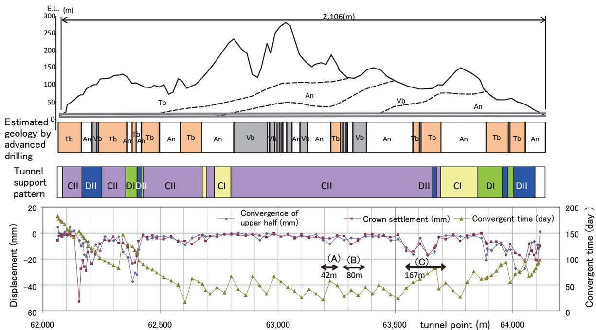
**Fig. 1** Geology, displacement and three repaired area (A, B, C) of the studied tunnel
