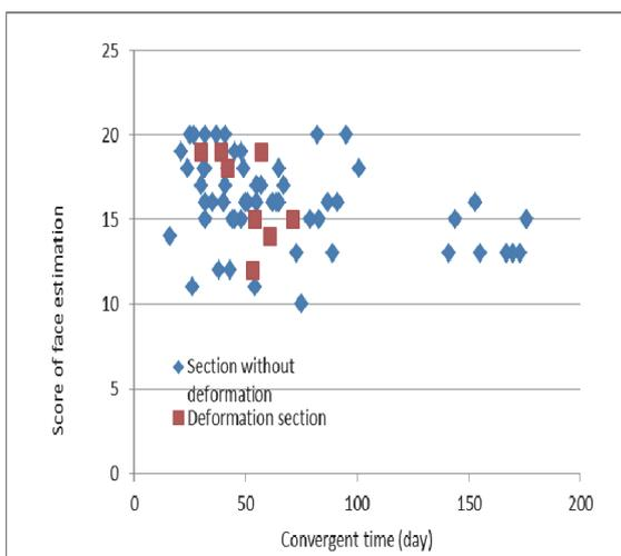
**Fig. 5** Relation between convergent and score of face estimation in non-inverted part
