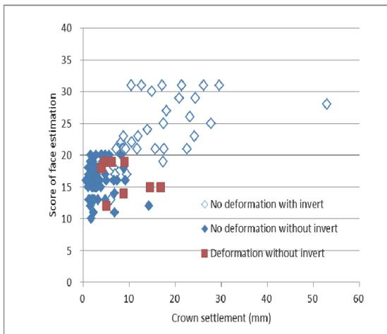
**Fig. 3** Relation between crown settlement and score of face estimation
