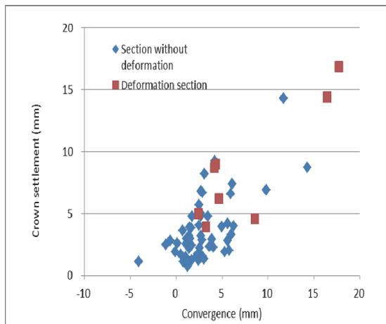
**Fig. 4** Relation between convergence and crown settlement of non-inverted part
