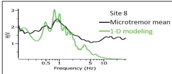
Fig.8 Comparison of empirical and theoretical transfer functions at site 8, by considering the Karaj basement (>2500 m/s) at depth of 2200 m.
