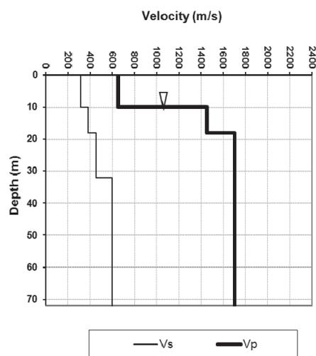
Fig.4 Shear wave velocity profile obtained from downhole test at A09 borehole (site 8).
