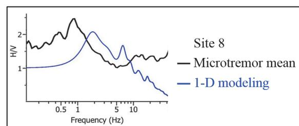
Fig.5 Comparison of empirical and theoretical transfer functions at site 8, by considering the engineering bedrock (>760 m/s) at depth of 85
