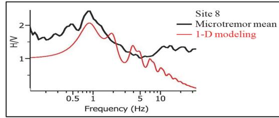
Fig.7 Comparison of empirical and theoretical transfer functions at site 8, by considering the geology bedrock (>1300 m/s) at depth of 230 m.
