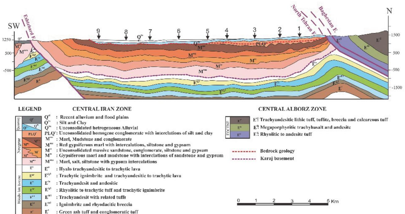
Fig. 9 Two-dimensional model of Karaj subsurface structure (Derived from the geological map with changes)
