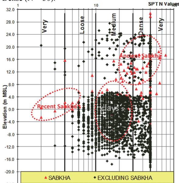
**Fig. 5: Plot of SPT vs Depth**
