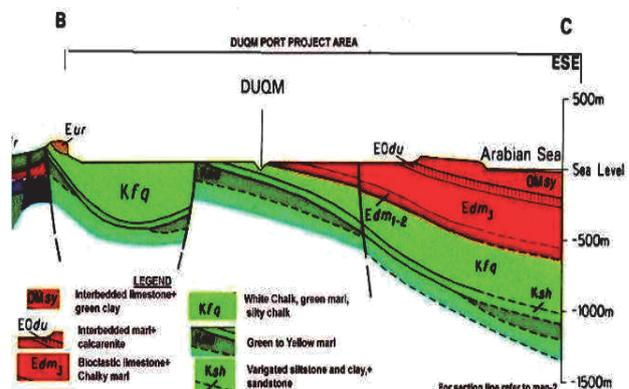
Fig. 3: Geological cross section across Duqm area (Platel et al., 1992)
