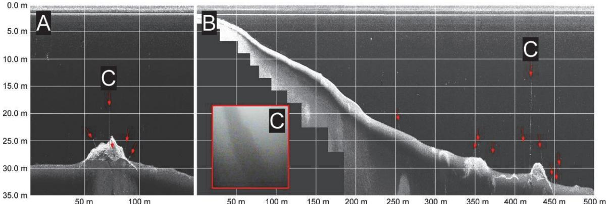
Fig. 4 (A and B) Vertical acoustic profiles of 455 kHz shown in Fig. 2 and 3. Red arrows indicates trees standing on the lake floor. (C) A trunk of tree observed by underwater camera.
