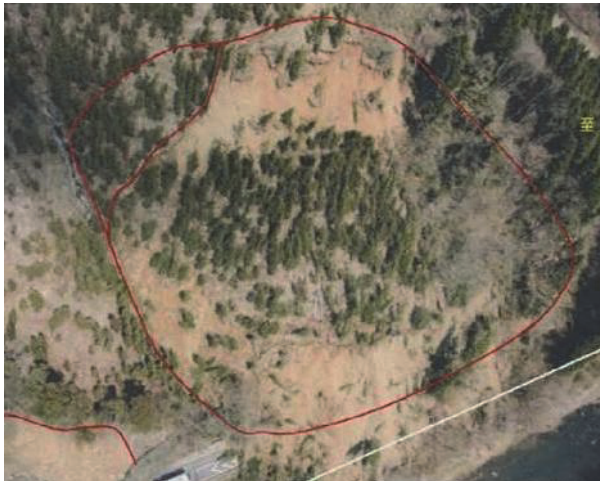
Photo 14 A case of deep-seated landslide in the Mesozoic schist area
