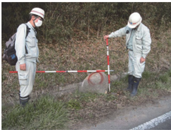
Photo 7 A case of rockfall of a corestone remained from weathering in the Mesozoic granodiorite area
