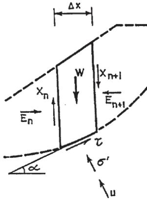
Fig. 2 Stresses and Forces Acting on a Typical Slices.
