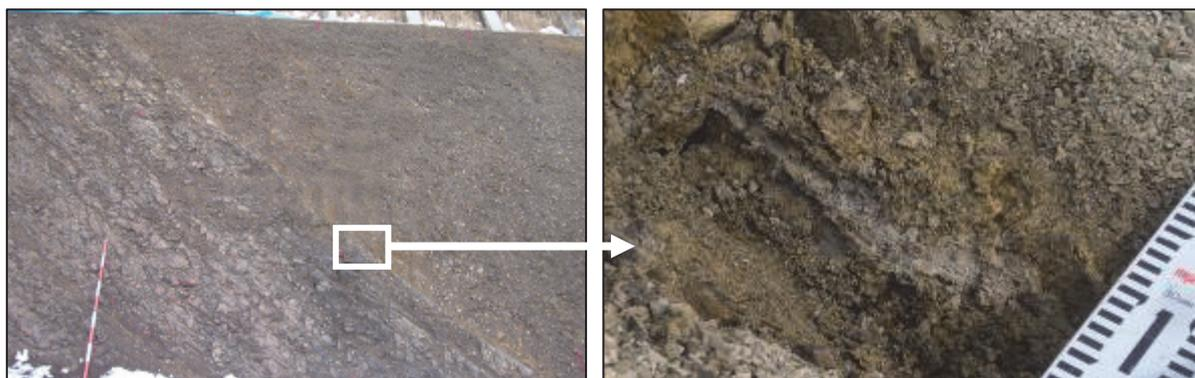
Photo. 4 Boundary of the shale layer
