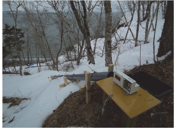
Fig. 4 An installed wire-type extensometer.
