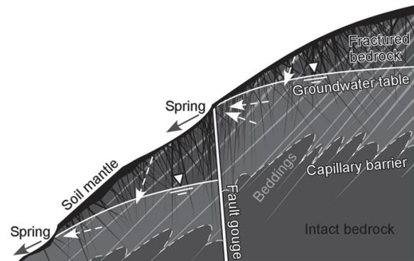
Fig. 5. Schematic illustrating bedrock aquifer system separated by high-angle impermeable fault gouge. Quick piston flow due to rainfall infiltration through fissures recharges the bedrock groundwater. The bedrock aquifer drains groundwater by overflowing of the subsurface dam as persistent spring discharge.
