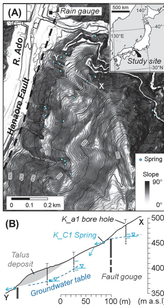
Fig. 1 Topographic map of the study site (A) and hillslope profile surveyed (B). Three borings were drilled on the profile and used as observation well with a screen for depths represented by broken lines. Groundwater tables are indicated by max, mean and min levels during 2013–2014.
