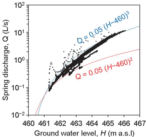
Fig. 4. Correlation between upslope groundwater level in bedrock and discharge from spring (black dots). Blue and red curves indicates a cubic and a quadratic function to explain the overflow drainage from bedrock aquifer.
