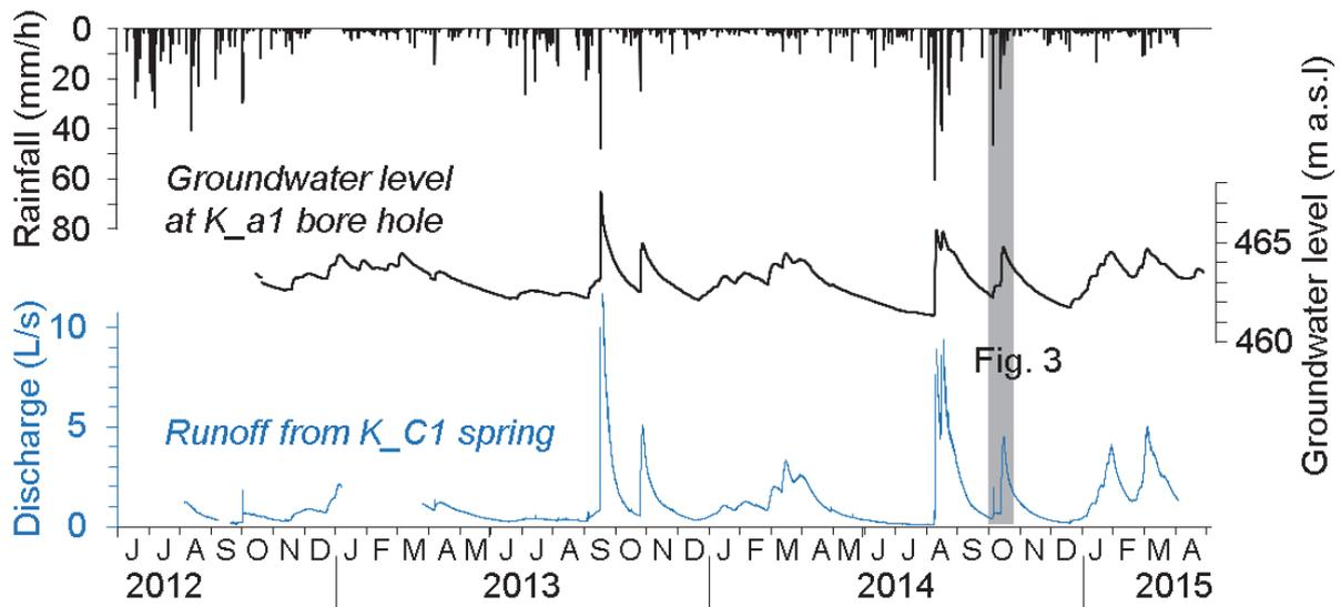
Fig. 2 Hydrograph observed at a bedrock spring (blue) and groundwater response in bedrock (black).
