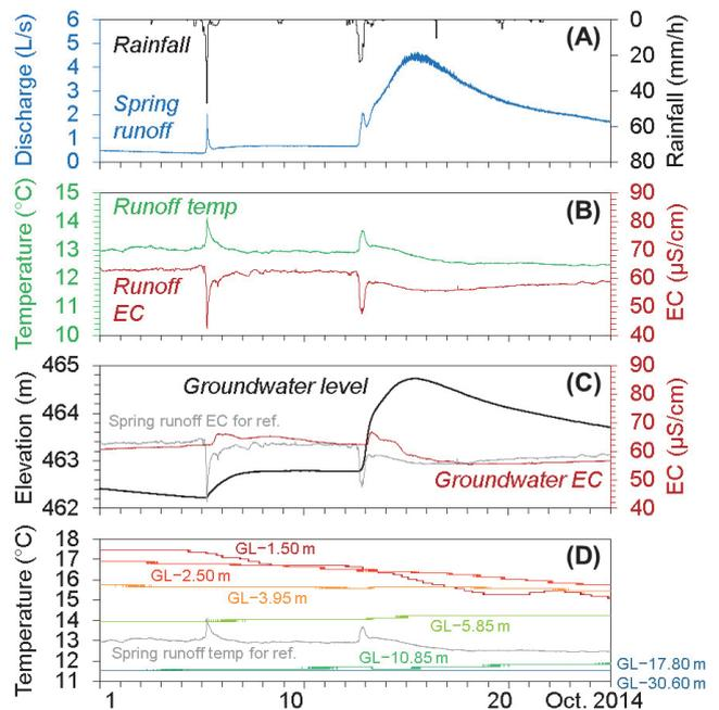
Fig. 3. Typical responses in spring runoff and groundwater level for intense summer rainfall events. (A) Rainfall and discharge at K\_C1 spring. (B) Responses in temperature and electrical conductivity (EC) of the runoff water from the spring. (C) Responses in groundwater level and EC at the K\_a1 bore hole. EC of spring runoff (grey) is indicated for reference. (D) Changes in temperature in the depth profile at the K\_a1 bore hole. Temperature of spring runoff (grey) is indicated for reference.
