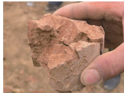
Fig.4 Mirror surface and striation in drill cores
