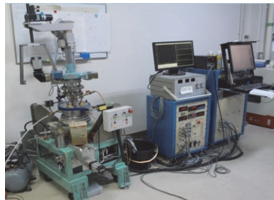
Fig. 4 Portable ring shear apparatus ICL-1 with its instrument box, monitoring box and control box
