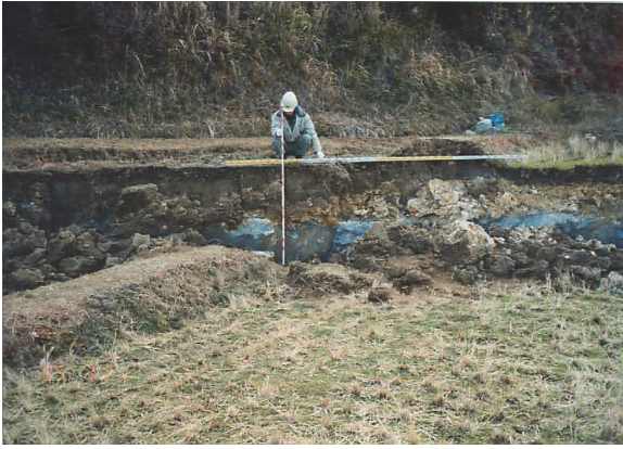
Photo 1. Fresh rupture scarp emerged along the Nojima fault on Awaji Island at the 1995 Kobe earthquake.
