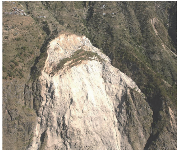
Photo. 4 Failure in deep-seated old landslide
